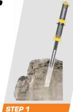
Insert half of the total length of the wedge and use the Yamamoto splitter to split.
